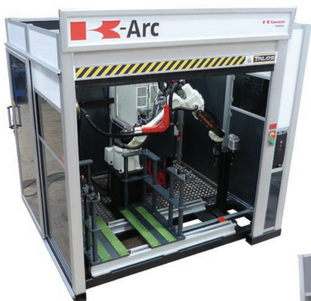
Robotic CMT welding cell for veterinary cages
